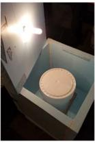
and adjusting wattage of the bulb. Alternatively, you can hook the light to a dimmer and adjust as needed to reach the desired temperature.
