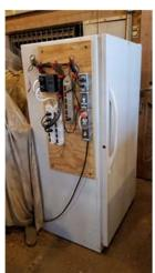
Another method is the use of an electronic controller that monitors a set temperature and turns a heater "on" or "off"—can be an incandescent bulb(s) or other heater. Often these are used in conjunction with a decommissioned
